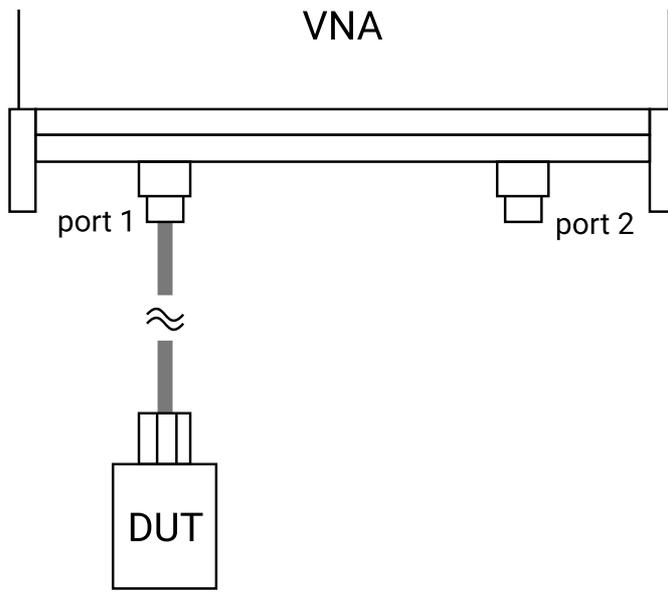
Connect device under test to Port 1 to carry out  $S_{11}$  measurements.
