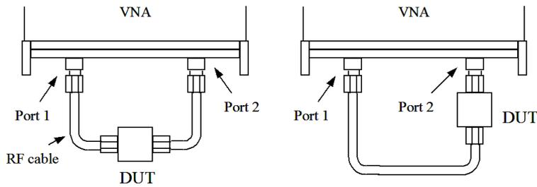
Connect DUT between Ports 1 and 2 to carry out S<sub>21</sub> measurements. For best results use the arrangement shown on the right
