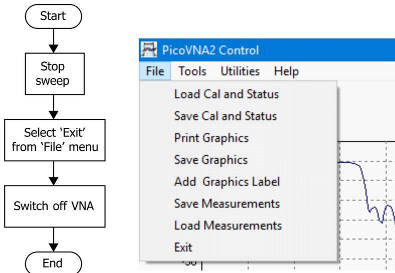
Formally closing down the software saves the current calibration
