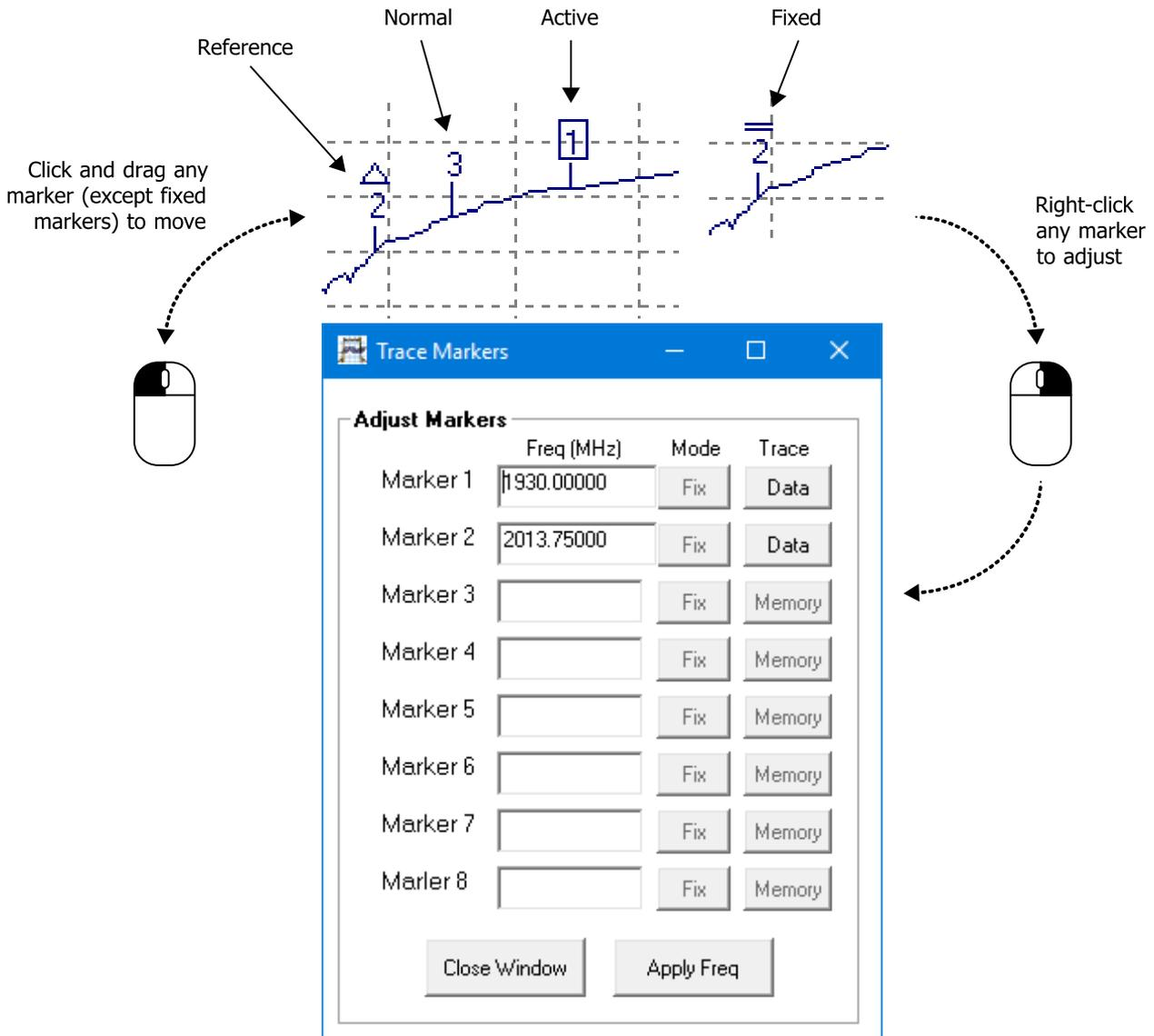
Change the marker type by right-clicking on any marker on the active channel. Note that only the reference marker can be fixed.
