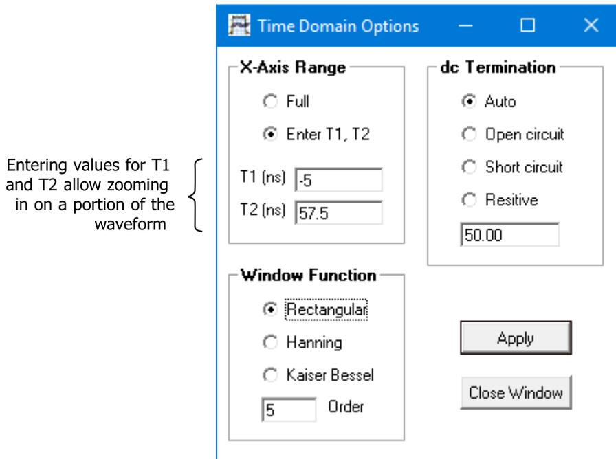
Entering values for T1 and T2 allow zooming in on a portion of the waveform
