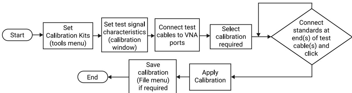
Instrument calibration sequence. This loop is fully automated when using an E-Cal module.
