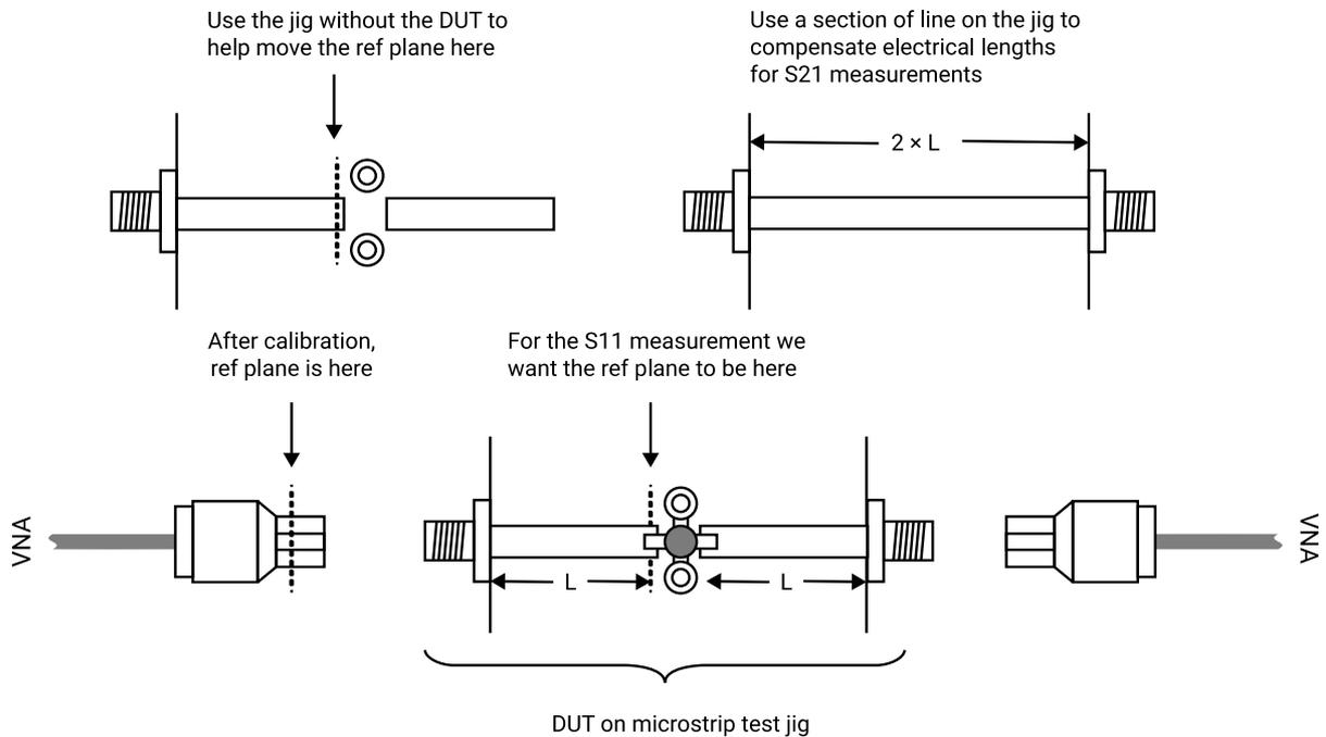
Correcting  $S_{21}$  and  $S_{11}$  phase measurements. Reference plane extension corrects  $S_{11}$  measurements and normalization to a test line corrects  $S_{21}$ .
