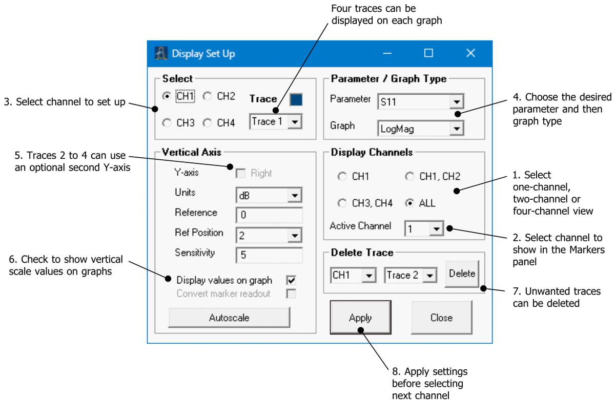
The Display Set Up window is used to set up the measurements display
