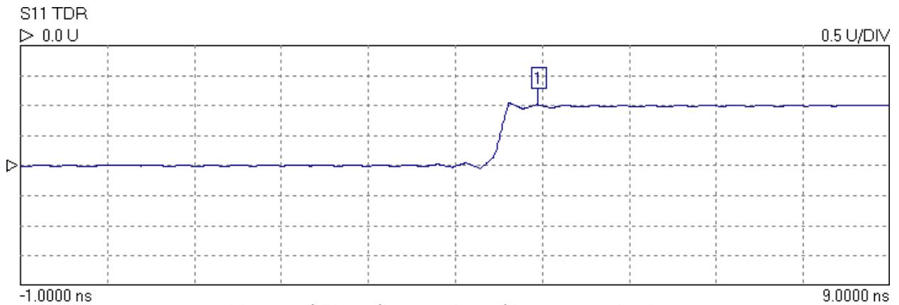
Measured 50 cm line terminated in an open circuit.
