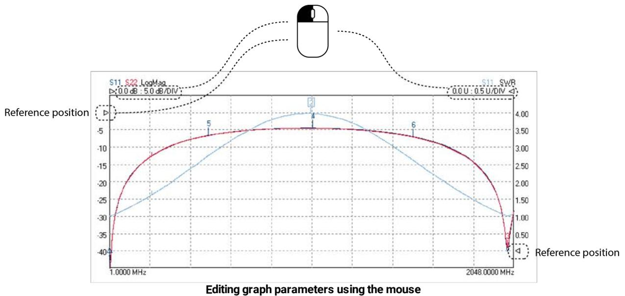
The figure above shows how the mouse can be used to quickly adjust reference position, reference value and vertical scale sensitivity for the graph. Hover the mouse pointer over the number, or the reference position triangle, then click and drag to adjust the indicated values up and down. To type the values for reference value and vertical scale, hover the mouse over the number, right-click and type. To save the value, press enter or left-click.
