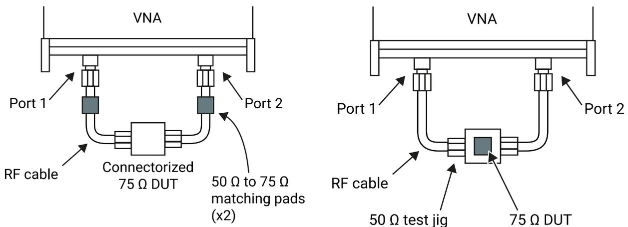
Impedance matching pads can be used to measure a connectorized device. Use external matching pads and calibrate with a 75  $\Omega$  calibration kit.
