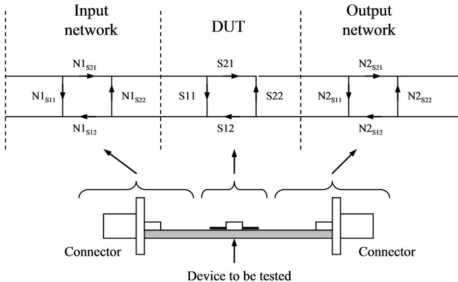
De-embedding allows the effects of the test jig's input and output networks to be removed.
