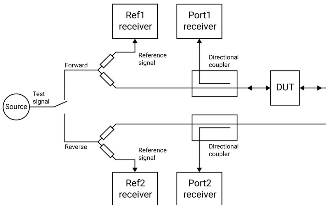
Simplified vector network analyzer block diagram
