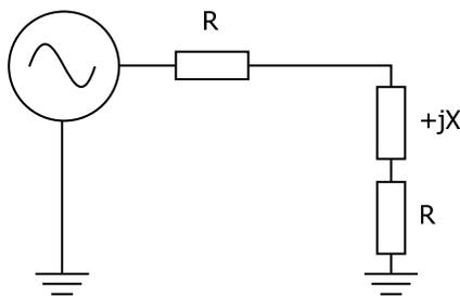
Matching network,  $-jX$ , ensures all power is transmitted to the load.
