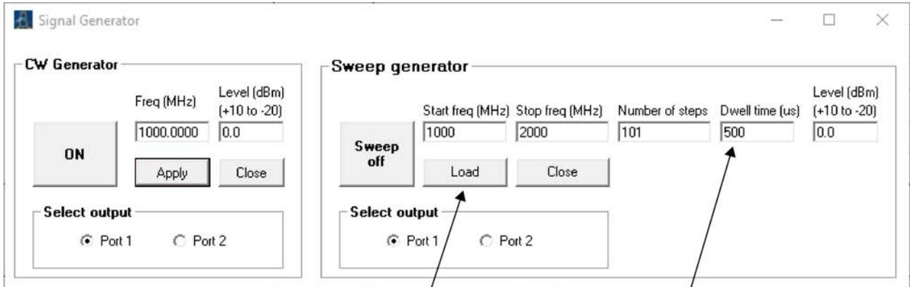
Before using the sweep mode, load the sweep plan
