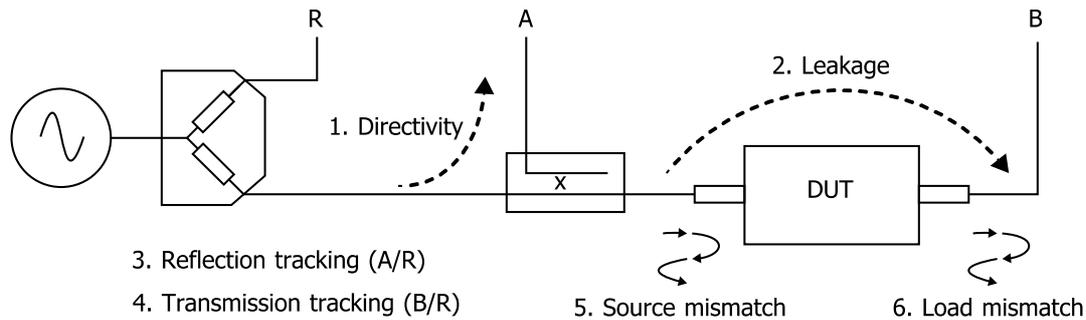
Six key sources of errors in forward measurement.
