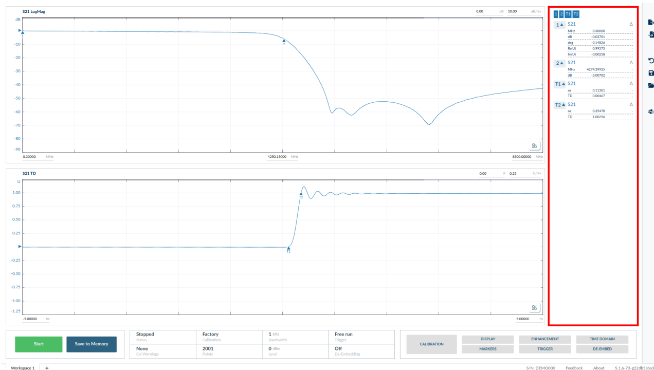
Figure 4.17: Highlights the marker readouts panel, here showing a selection of frequency domain and time domain marker readouts.
