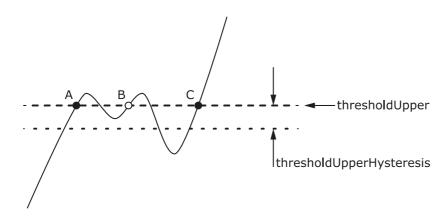
Hysteresis – The trigger fires at A as the signal rises past both thresholds. It does not fire at B because the signal has not passed the hysteresis threshold. The trigger fires again at C after the signal has dipped below the hysteresis threshold and risen past both thresholds.
