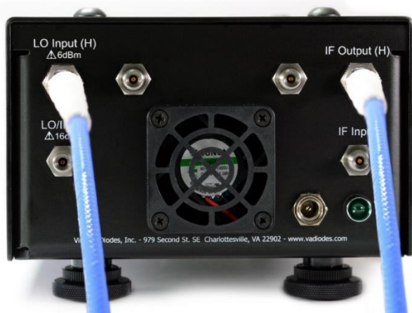
Figure 3: Block Down-Conversion – High Frequency LO Input Proper configuration details for down-conversion using the high frequency LO input port are shown. The IF Input Port is not used.
