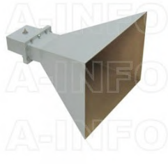
LB-OH-650-15-C-SF Octave Horn Antenna 1-2GHz 15dB Gain SMA Female
