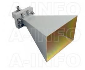
LB-OH-159-15-C-TF Octave Horn Antenna 4-8GHz 15dB Gain TNC Female
