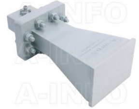
LB-OH-159-10-C-SFSPO Octave Horn Antenna 4-8GHz 10dB Gain SMA Female
