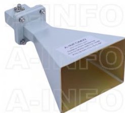
LB-OH-112-15-C-SF Octave Horn Antenna 6-12GHz 15dB Gain SMA Female
