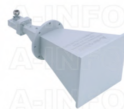
LB-65180-20-C-NFSPO Multi Octave Horn Antenna 6.5-18GHz 20dB Gain N Type Female
