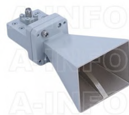
LB-65180-10-C-SF Multi Octave Horn Antenna 6.5-18GHz 10dB Gain SMA Female
