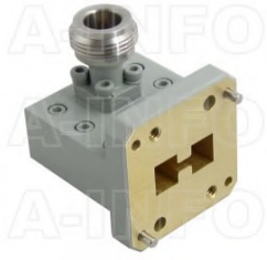
650DRWCAN_Cu Right Angle Double Ridge Waveguide to Coaxial Adapter 6.5-18GHz WRD650 to N Type Female
