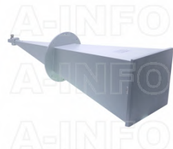
LB-60180-25-C-NFSPO Multi Octave Horn Antenna 6.0-18.0GHz 25dB Gain N Type Female
