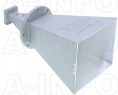
LB-60180-20-A Multi Octave Horn Antenna 6-18GHz 20dB Gain Double Ridge Waveguide Interface
