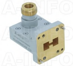
650DRWHCAN_Cu Right Angle High Power Double Ridge Waveguide to Coaxial Adapter 6.5-18GHz WRD650 to N Type Female
