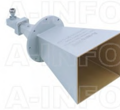
LB-58160-20-C-NF Multi Octave Horn Antenna 5.8-16GHz 20dB Gain N Type Female
