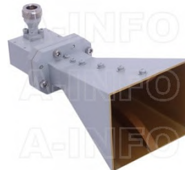
LB-475110-10-C-NF Multi Octave Horn Antenna 4.75-11GHz 10dB Gain N Type Female
