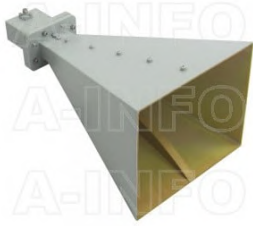
LB-3582-15-C-SF Multi Octave Horn Antenna 3.5-8.2GHz 15dB Gain SMA Female
