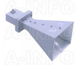
LB-3582-10-C-SF Multi Octave Horn Antenna 3.5-8.2GHz 10dB Gain SMA Female
