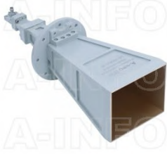
LB-180400-25-C-2.4F Multi Octave Horn Antenna 18-40GHz 25dB Gain 2.4mm Female
