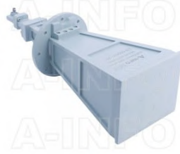
LB-180400-25-C-2.4FSPO Multi Octave Horn Antenna 18-40GHz 25dB Gain 2.4mm Female
