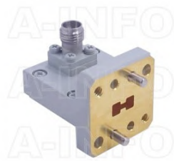
180DRWCA2.4_Cu Right Angle Double Ridge Waveguide to Coaxial Adapter 18-40GHz WRD180 to 2.4mm Female
