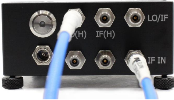
Figure 4: Block Up-Conversion Proper configuration details for up-conversion are shown. The IF Output (H) Port is not used.
