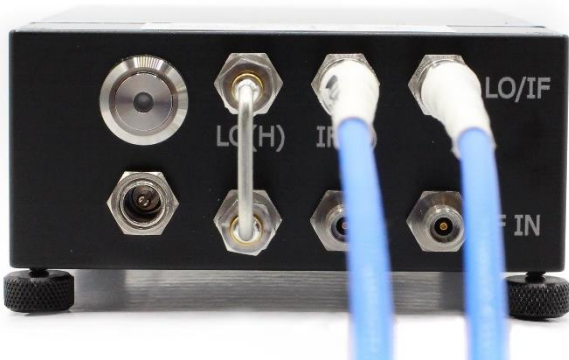
Figure 2: Block Down-Conversion – Low Frequency LO Input
