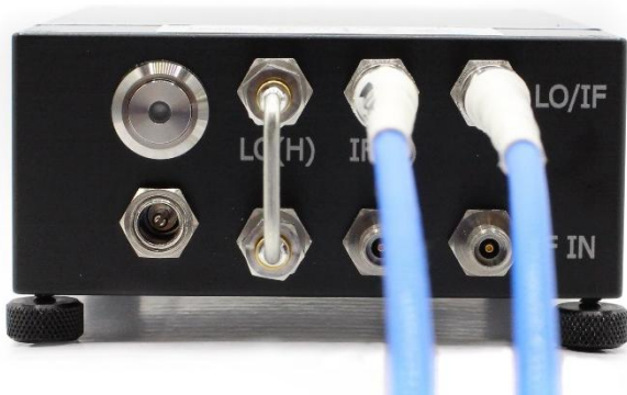
Figure 2: Block Down-Conversion – Low Frequency LO Input
