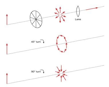
Radial polarization can be changed to azimuthal one by rotating segmented waveplate at 45 degrees. Direction of radial polarization becomes the opposite one by rotating the waveplate at 90 degrees.
