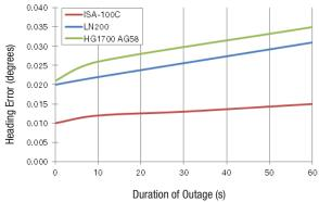
When SPAN is in RTK mode. O seconds outage on land vehicle application. RMS, incremental error growth from steady state accuracy. Computed with GPS, RTK trajectory using Waypoint Inertial Explorer. 1. 2. 3.
