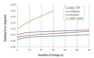
When SPAN is in RTK mode. Based on O seconds outage duration.
