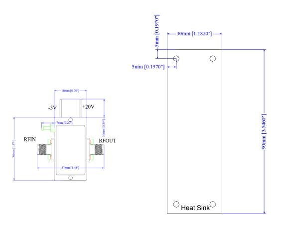
\*\*\*Heat Sink and cooling fan required during operation\*\*\*
