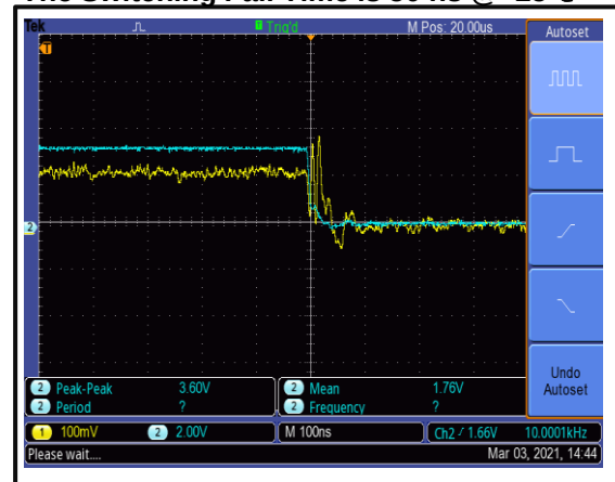
The Switching Fall Time is 50 ns @+25°C
