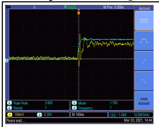
The Switching Rise Time is 100 ns @+25°C
