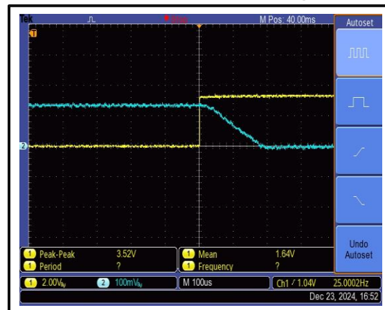
The Drains Closure Time is 200us @+25°C
