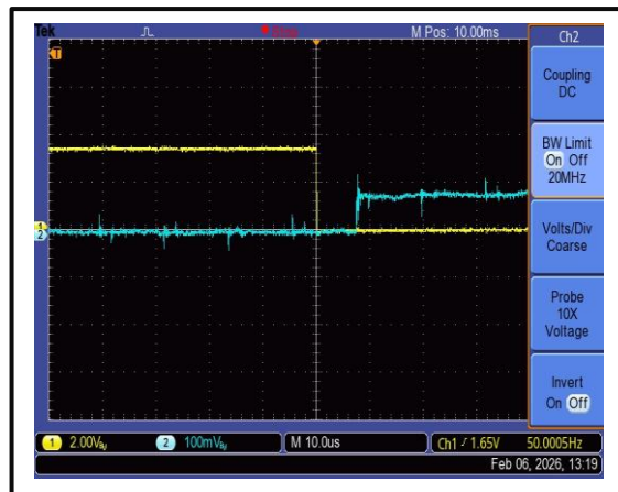
The RF Switch On Time is 8 us @+25°C
