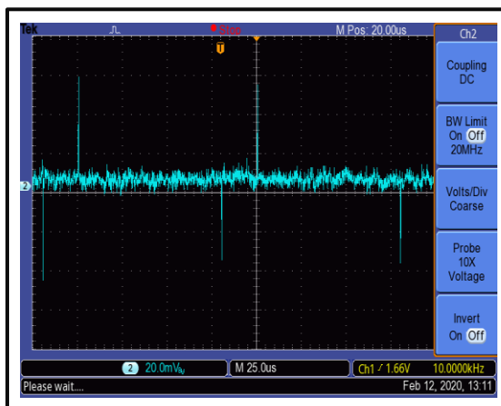
Video Leakage (Peak to Peak) @+85°C
