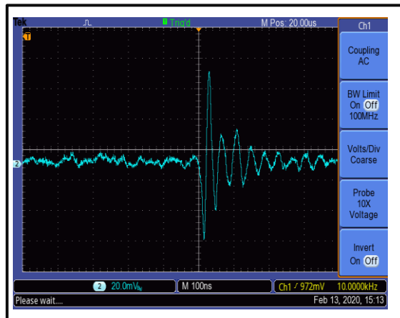
Video Leakage (Peak to Peak) @-40°C
