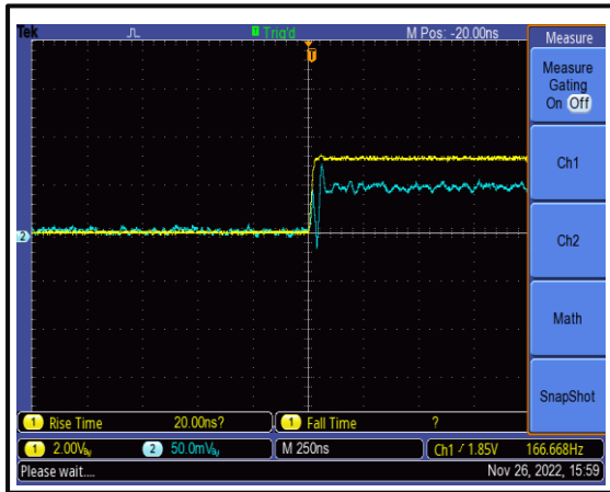
The Switching Rise Time is 100 ns @+25°C
