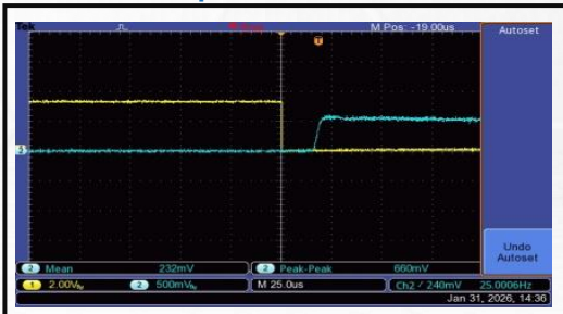
The Drains Open Time is 100 us
