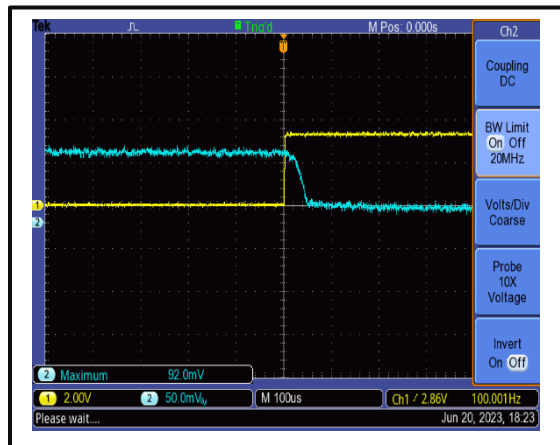
The Gate-Enable Rise Time is 50 \mu s @+25°C
