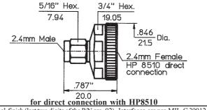
Dimensions shown are inches over millimeters. Standard units have stainless steel finish (last two digits of the P/N are -02). Interfaces are per MIL-C 39012, MIL-C-87104/2, MIL-C-3643, MIL-STD-348, IEC-169-7, IEC-457-2, DIN 47 223, DIN 47 226, DIN 47 298, where applicable. For details please refer to the beginning of this section.
