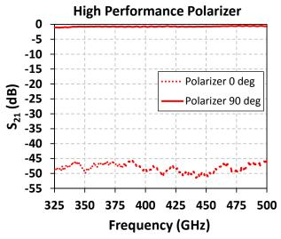
Transmission loss < 1dB Parallel isolation > 45 dB
