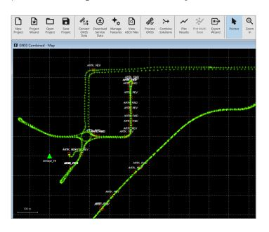
GrafNav refines your raw GNSS data by resampling, concatenating and splicing, processing forward and reverse in time then combining the results to generate a final trajectory. Moving baseline processing is supported, as well as heading determination using two fixed antennas on the same moving vehicle:
