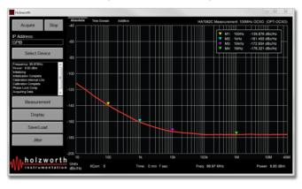
The highly intuitive HA7062C interface is a driver-free, MATLAB™ Runtime based GUI that will operate on any standard PC. No MATLAB™ license required.
