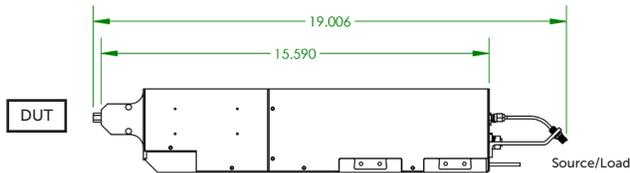
For best on-wafer operation DELTA tuners are equipped by default with male connectors DUT-side and female connectors Source/Load side. Different Configurations are possible on specific customer requests
