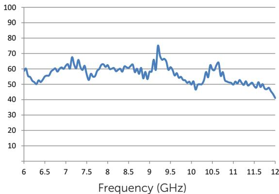
Insertion Loss (dB) (Probe withdrawn)
