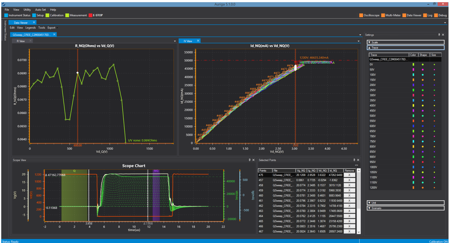
Auriga software interface displaying dynamic On-resistance measurement
