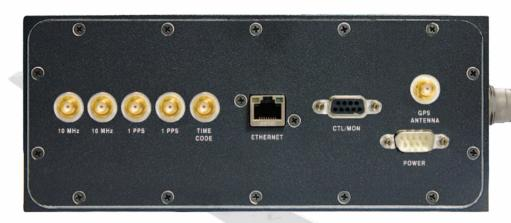
The NanoSync IV is a small form factor GPS Position, Navigation, Time (PNT) and Frequency reference system that provides multiple reference outputs and includes support for NTP & PTPv2 IEEE 1588-2008. The NanoSync IV has a Rubidium oscillator and is equipped with a SAASM receiver (Rockwell-Collins MPE-S GB-GRAM or Trimble Force 22E MRU) for military users. The NanoSync IV is packaged in a small, rugged enclosure ideally suited for embedded electronic warfare applications.
