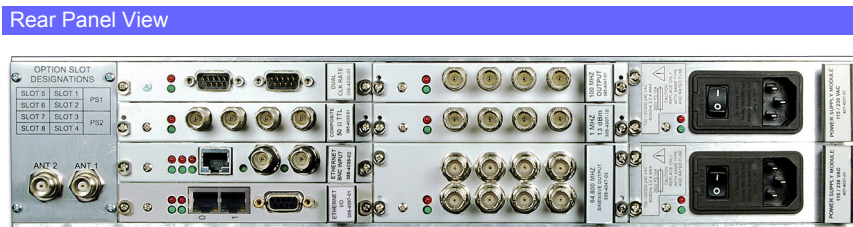
8 Input/Output Hot-Swappable Option Module Slots
