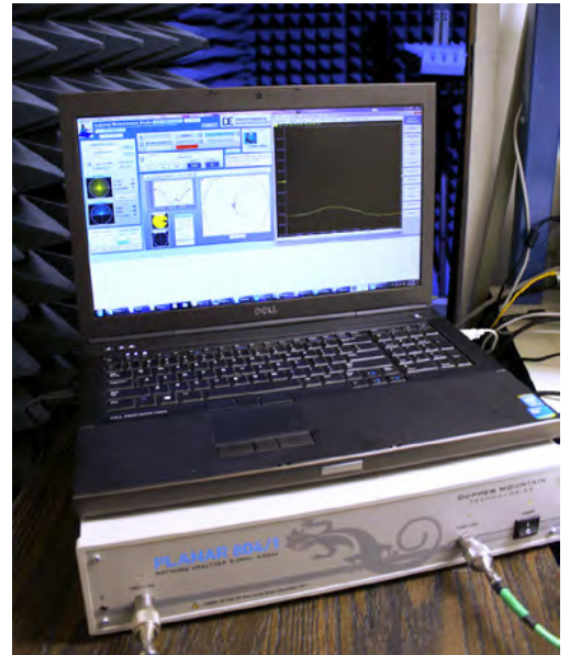
Left: the AUT is tuned at 2420 MHz Right: the VNA and DAMS software operate in tandem on a PC
