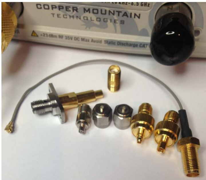
SMA to RF switch, SMA to U.FL (both sexes), SMB, SMA bullet and SMA to U.FL short cable, and a Vector Network Analyzer.
