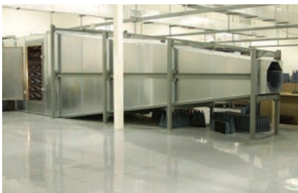
▲ Fig. 1 A typical tapered anechoic chamber.
