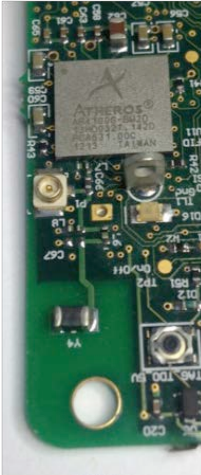
U.FL connector sits on a stub with the same length as the trace to the WiFi module. In production, omit the U.FL connector.
