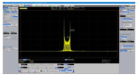
All PicoScope 9400 Series oscilloscopes can calculate real, imaginary and complex Fast Fourier and Inverse Fast Fourier Transforms of input signals using a range of windowing functions. The results can be further processed using the math functions. FFTs are useful for finding crosstalk and distortion problems, adjusting filter circuits, testing system impulse responses and identifying and locating noise and interference sources.
