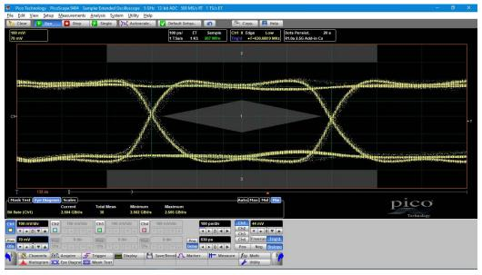
PicoSample 4 has a built-in library of over 130 masks for testing data eyes. It can count or capture mask hits or route them to an alarm or acquisition control. You can stress-test against a mask using a specified margin, and locally compile or edit masks.
