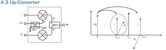
An up converter is a mixer application which takes a low frequency small signal IF input, and a high frequency large signal LO input and mixes the signal together to produce a high frequency RF output. The fundamental 1IFx1LO outputs present at the RF port are the  $f_{LO-IF}$  and  $f_{LO+RF}$  tones. An up conversion can select either the  $f_{LO-IF}$  or the  $f_{LO+IF}$  tones. The above illustration shows both up converted sidebands with either an I or Q port input signal.
