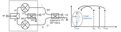
An image reject mixer is a mixer which rejects the down converted image frequency from the IF output. Image reject mixers are constructed using an external quadrature hybrid attached to the I and Q (i.e., IF) output ports. Using the external IF quadrature hybrid, one can select whether the upper sideband or lower sideband signal is suppressed with respect to the LO signal.
