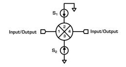
A vector modulator is a device that can modulate an input signal's amplitude and phase. Similar to using a double balanced mixer as a phase modulator or phase shifter, an IQ mixer can be used as a vector modulator. An IQ mixer can be used as a vector modulator by inputting DC current into both the I and Q ports.
