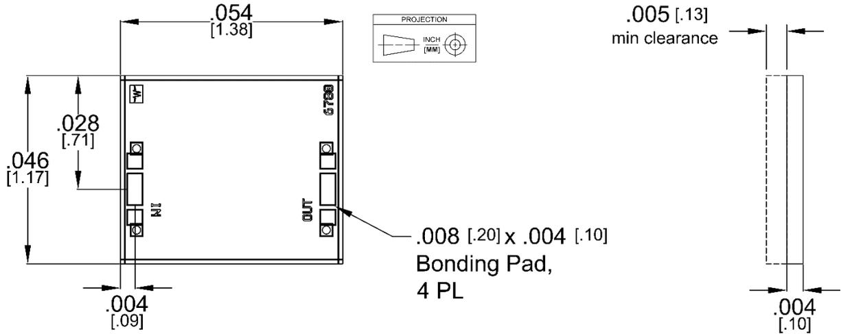
1. CH Substrate material is 0.004 in thick GaAs.
