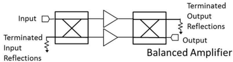
In a balanced amplifier, the poor return loss of an amplifier is compensated for with a quadrature hybrid. In this application, the reflections from the input or output are collected at the isolated port of the quadrature hybrid and terminated.
