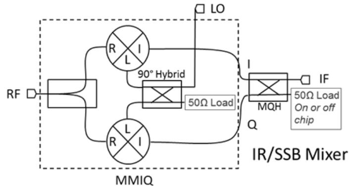
The primary application for the MQH and MQS series is as IF or LO quadrature signal splitter/combiners. They can be used in combination with the MMIQ series of IQ mixers to create broadband single sideband and image reject mixers. Either 90° Splitter/Combiners or quadrature hybrids can be used as the IF hybrid, but if a 90° Splitter/Combiner is used only one sideband (or image) is accessible, whereas if a quadrature hybrid is used then both sidebands are accessible.
