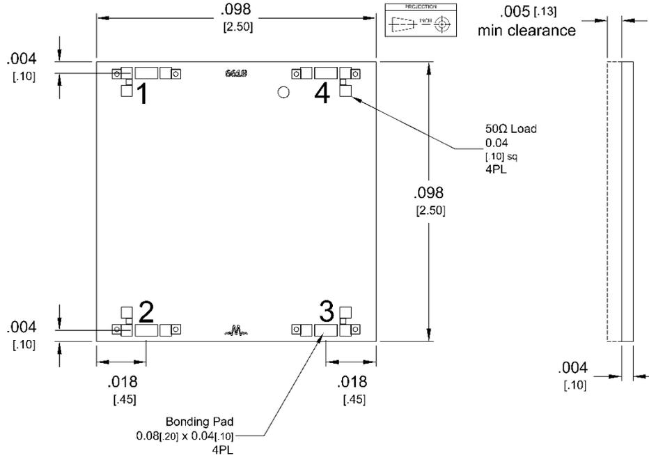
1. CH Substrate material is 0.004 in thick GaAs.
