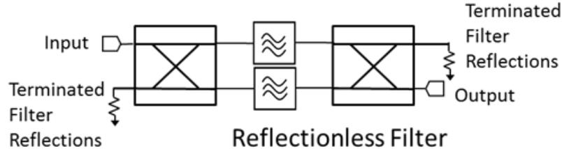
Similar to a balanced amplifier, a reflectionless filter will terminate reflections that are out of band for a filter (but in band for the quadrature hybrid) at the isolated port.
